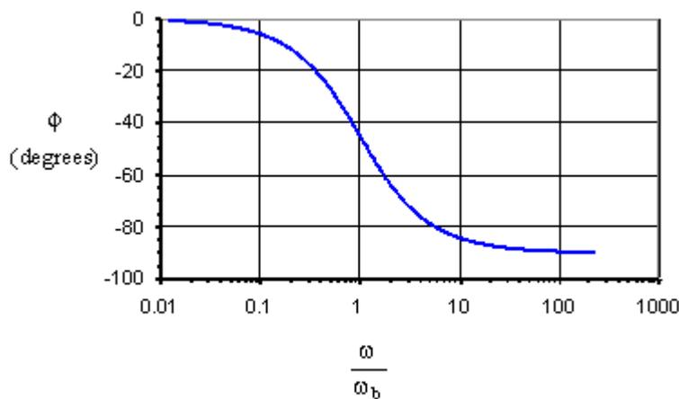
The phase angle is zero (no phase shift) for very low frequencies, but falls off rapidly. Even at the corner frequency, the phase shift is significant, i.e.  $-45^\circ$ . For high frequencies the phase shift asymptotes to  $-90^\circ$ .
