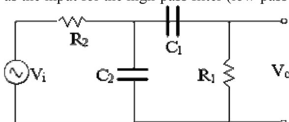
The left portion of the schematic diagram represents the low-pass filter, and the right portion represents the high-pass filter.
