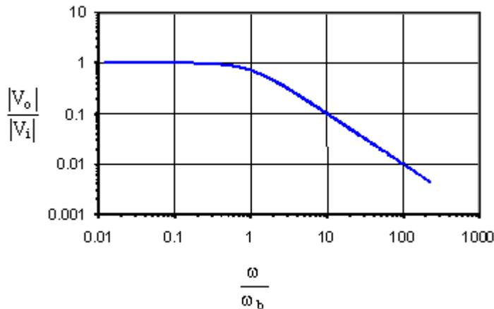
Notice how the low frequencies pass relatively unaffected, but the high frequencies get attenuated. Also notice that the drop-off with frequency looks linear on this log-log plot.
