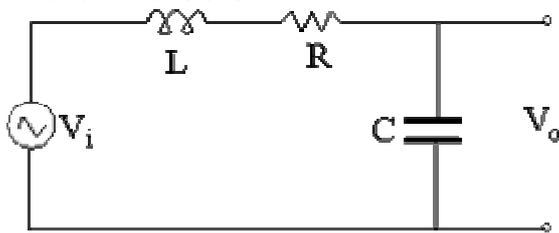
In this case, it turns out that the filter behaves as a *second-order* low pass filter.
